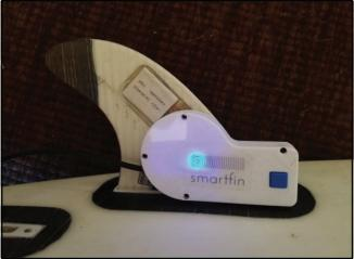
Press the start button on the charger. The charger will flash blue and red, then stay blue if properly aligned. The LED on the fin will turn from Red to Green when the fin is ready to surf, and the green LED will turn off when the fin is fully charged. The fin will hold its charge without use for one week.
